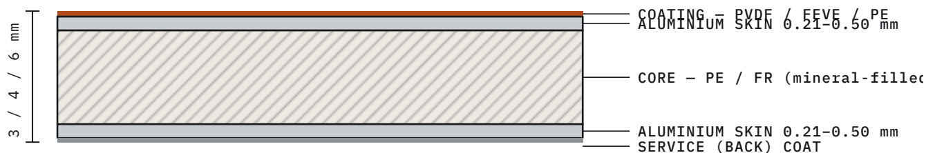
SECTION THROUGH COMPOSITE PANEL (NOT TO SCALE)
